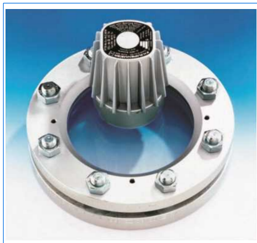
illuminated sightglass unit, consisting of sightglass to DIN 28120, DN 150, PN 10, with mounted LUMIGLAS light fitting, 30 V, 20 W, 2Ex d e IIC T4 Gb, Ex t IIIC T130°C Db IP67, Ex II 2 G + D, with anti-dazzle shield "B", in version "view and light through one assembly"
