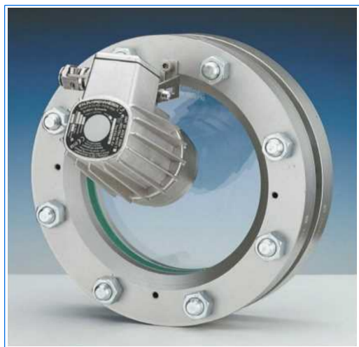
LUMISTAR illuminated sightglass unit, consisting of sightglass to DIN 28120, DN 80, PN 10, with mounted LUMIGLAS light fitting, 24 V, 20 W, Ex d IIC T5 Gb, Ex t IIIC T95°C Db IP 67, Ex II 2 G + D
