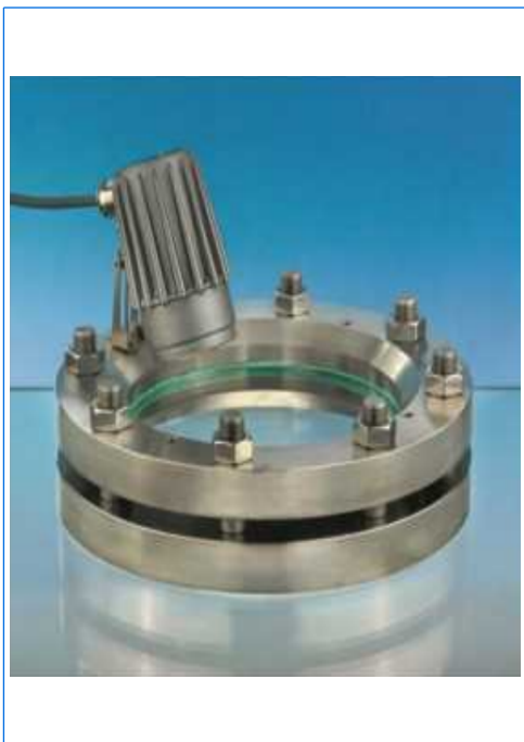
Complete assembly of sightglass fitting to DIN 28120, DN 125, PN 10, with glass disc of toughened sodium silicate to DIN 8902, fitted with LUMIGLAS sightglass light fitting, tilting hinge fixation
