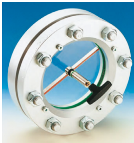
Circular sightglass, DN 150, PN 0, with glass disc in sodium silicate to DIN 8902 and wiper of the series W, wiper blade in silicone
