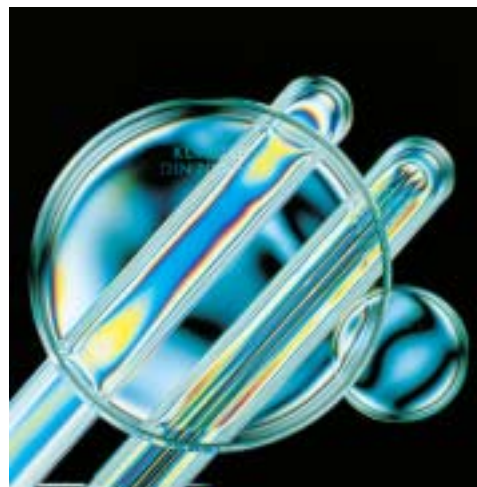
Stress-optical view of thermally prestressed circular and long gauge glasses in polarized light
